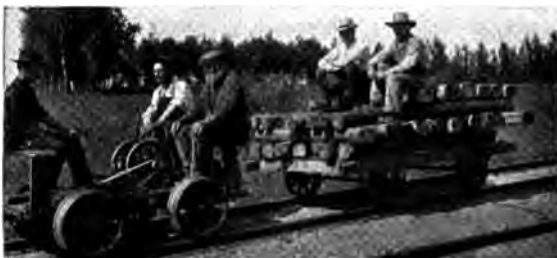
Our 3 Horse Engine pulling a push car, 30 ties, 5 men up grade and made a speed of 10 miles per hour.
